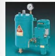
To pre filter these products through a 3 Micron filtration system ensuring that the products are cleaned to meet the industries high ISO oil cleanliness standards.
